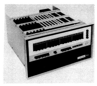
The Microdata 1600 is rack-mountable or, with the proper cover, may be placed on a desk or table top. The processor features the capability for emulating other systems as well as for developing new ones through microprogramming by the manufacturer or the user
