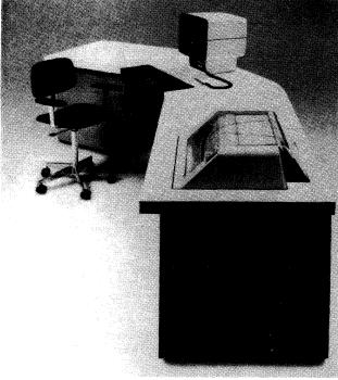
All five of the current Magnuson processors are housed in this compact cabinet, which contains the CPU, console display and keyboard, up to 4 megabytes of memory, and up to 8 I/O channels. Larger configurations require an add-on Expansion Module that adds 26 inches to the overall cabinet width. The optional Console Printer is in the foreground.
