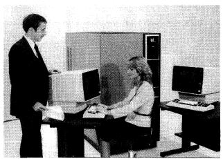
The IPL 4400 Series systems have from 4 to 16 megabytes of main memory, support 6 to 10 I/O channels, are field-upgradable, and feature better price/performance than comparable IBM 4300 Series processors.
