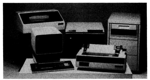
The System Ten Model 320 shown here includes a wide range of the standard peripheral units available. The Model 320 processor is flanked by a 300 lpm, 132 column printer and a 20 megabyte cartridge disk. The CRT shown is the Model 85 Display Unit and the adjacent printer is the 180 cps, matrix serial model.
