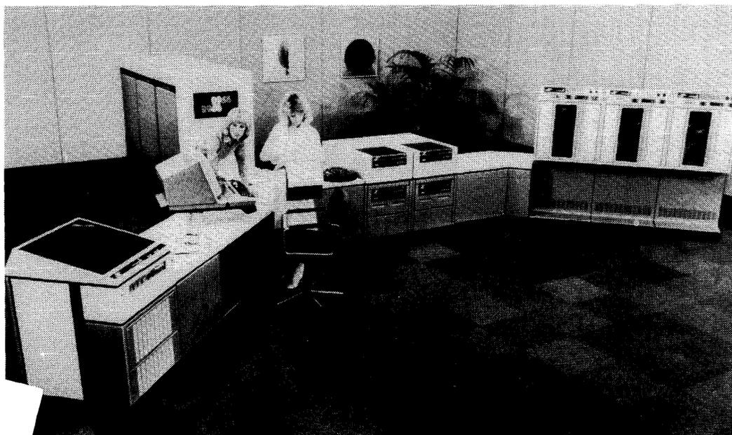
*The new ICL 2956, above, like the ICL 2950, can be assembled in configurations that eliminate the need for raised flooring.*
