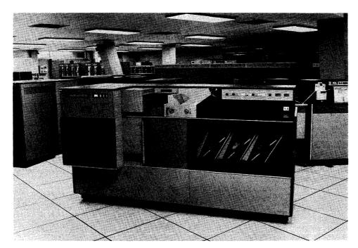
ICL's Universal Document Reader can be fitted with an optical mark and/or character reading head and from 3 to 12 stackers. Shown here is a 3-stacker model equipped for character reading.
