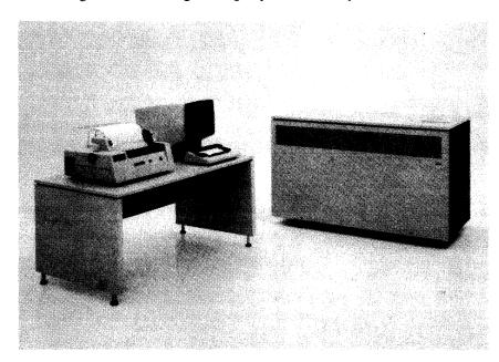
The smaller processor in IBM's new series, the 4331, can fit easily into an office environment. Shown here are the processor complete with its integrated adapters (right) and the system console with a hard-copy device. Missing from the photo are the two other elements needed for a basic 4331 configuration: a line printer and the new 3310 Direct Access Storage Device.
