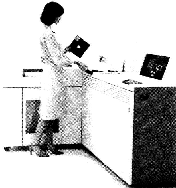
One of the more important units that is integral to the 5381 System Unit is the diskette magazine drive. This unit provides three functions: save/restore, diskette I/O, and CE servicing. The storage capacity of each diskette depends on type and formatting. Three types of diskette may be read by the unit in three different formats. Maximum capacity for the drive is 24 million bytes.
