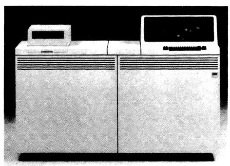
The System/38 Model 5XX is a packaged system consisting of the 5381 System Unit and its integral units. These units include the central processor, up to 2048K of main memory, a system console with keyboard and display screen, a diskette magazine drive, up to 387.1 megabytes of fixed disk storage, and a workstation controller. A printer (not shown in the photo) is optional.
