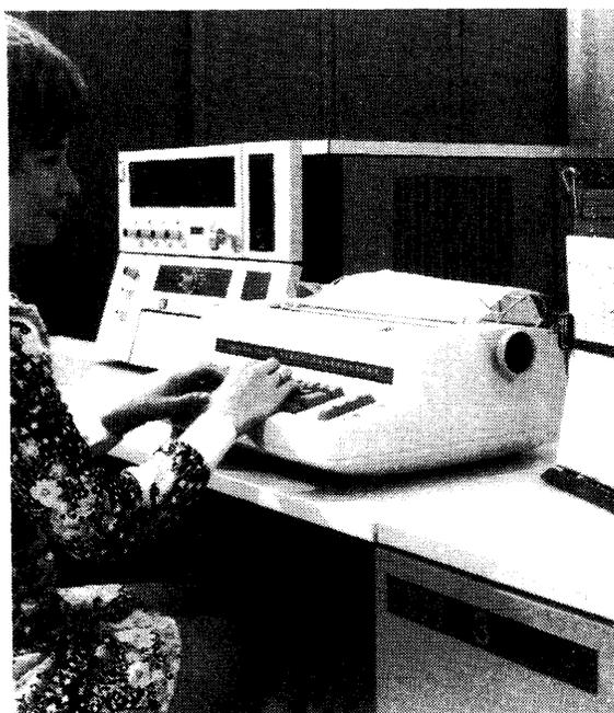
*The operator is working at the 5471 Printer-Keyboard, the alternate I/O device to the 3741 diskette Data Station for the new System/3 Model 8. A minimum configuration using the 5471, a 16KB central processor, a 2.46 MB disk drive, and a 100-lpm printer rents for \$1,599 monthly or sells for \$62,525.*
