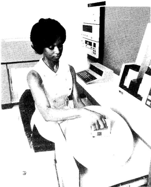
*In the System/3 Model 10, the compact 5444 Disk Storage Drive and its removable single-disk cartridge are conveniently housed in a drawer beneath the 5424 Multi-Function Card Unit.*
