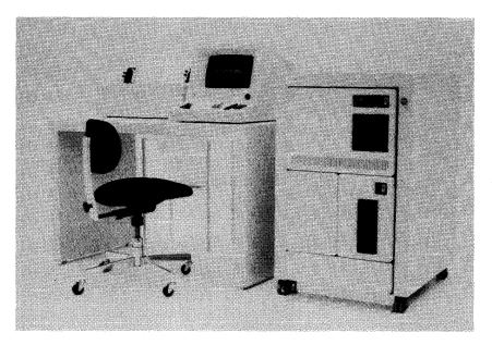
This small Series/1 configuration includes a low-boy rack enclosure housing the processor and a 4964 diskette unit. The table-top, 120 cps 4974 printer is shown at left. The display station in the photo is the 4979, one of two 1920-character display units offered with the Series/1.
