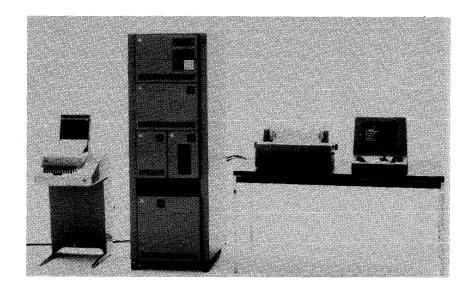
This Series/I configuration includes a 4997 rack enclosure with a 4955 processor mounted at the top and a 4959 input/output expansion unit below. The bottom half of the enclosure houses a 4962 disk storage unit, with a 4982 sensor I/O unit above and to the left, and a 4964 diskette unit to the right of the sensor unit. Also shown are the 4974 printer, 4979 display station, and a teletypewriter.
