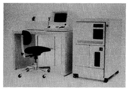
This small Series/I configuration includes a low-boy rack enclosure housing the processor and a 4964 diskette unit. The table-top, 120-cps 4974 printer is shown at left. The display station in the photo is the 4979, one of two 1920-character display units offered with the Series/I.
