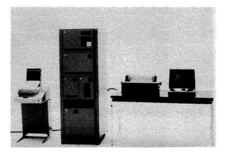
This Series/1 configuration includes a 4997 rack enclosure with a 4955 processor mounted at the top and a 4959 input/output expansion unit below. The bottom half of the enclosure houses a 4962 disk storage unit, with a 4982 sensor 1/O unit above and to the left, and a 4964 diskette unit to the right of the sensor unit. Also shown are the 4974 printer, 4979 display station, and a teletypewriter.
