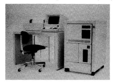
This small Series/1 configuration includes a low-boy rack enclosure housing the processor and a 4964 diskette unit. The table-top, 120-cps 4974 printer is shown at left. The display station in the photo is the 4979, one of two 1920-character-screen units offered with the Series/1.
