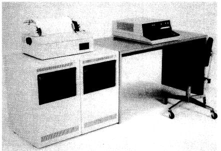
The 5110 Computing System shown includes the maximum complement of two 5114 Diskette Units, each housing two diskette drives. Each diskette can store up to 1.2 million characters of information, for a total on-line storage capacity of 4.8 million bytes. The keyboard/display houses the CPU with 16K, 32K, 48K, or 64K bytes of main memory and an optional magnetic tape cartridge unit. Two character printers are available with speeds of 80 and 120 cps, and both have upper and lower case capability.
