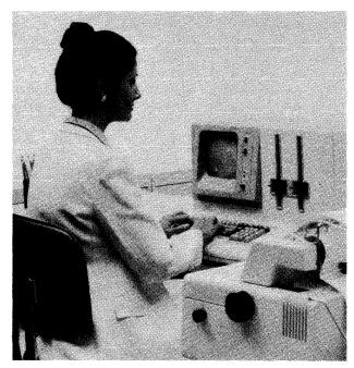
A typical IBM 5120 system, as shown above, features an integrated CRT display, two integrated floppy disk drives, and an attached typewriter-style keyboard. The 5103 Printer, seen in the foreground, is available as an option. System purchase prices range from \$5,680 (with Basic interpreter) to \$9,115 (with Basic/APL interpreters).
