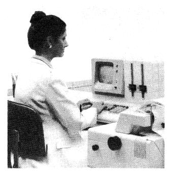
Dual integrated diskette drives and a larger display screen are the 5120's main functional advantages over its predecessor, the IBM 5110. In the foreground is the optional 5103 Printer.
