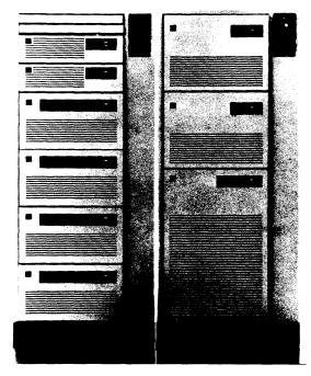
IBM's 9377 Model 90 is the high-end computer in the 9370 Information System family. This system features IBM's first air-cooled Thermal Conduction Module (TCM), and, according to the vendor, takes up little more space than two filing cabinets.
