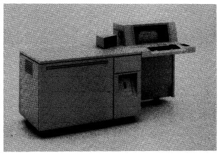
The highly integrated System/32 is a compact unit in a desk-sized cabinet. The appearance varies slightly from model to model, depending on the printer configured. The user has a choice of serial printers rated at 40, 80, or 120 cps and line printers rated at 50, 100, 155, or 285 lpm. Fixed-disk capacity can be 3.2, 5.0, 9.1, or 13.7 megabytes.
