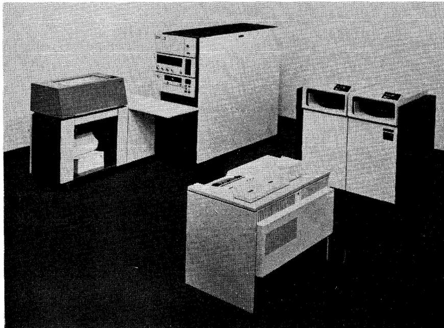
The System/3 Model 12, introduced in 1975, features the dual-drive 3340 Direct Access Storage Facility shown in the right background. In the foreground is a 3741 diskette data entry station, which is connected directly to the Model 12 processor for I/O. Beginning with the diskette-oriented Model 8 and continuing with the Model 12, it appears that the noble experiment IBM started in 1969 with the 96-column card is drawing to a close.
