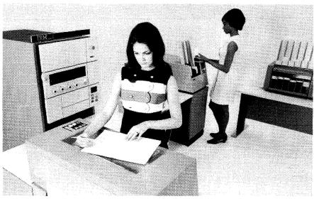
➤ access time as the Model 10 Processing Unit. However, the Model 8 main memory is the MOSFET semiconductor type, as used in the Model 15; memory is available in four steps from 16K bytes to a maximum of 64K, in increments of 16K. Logic circuitry in the processor is based on IBM's Monolithic Systems Technology like the rest of the System/3 product line.
