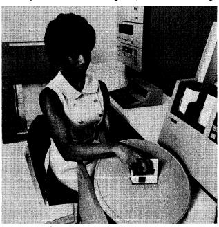
In the System/3 Model 10, the compact 5444 Disk Storage Drive and its removable single-disk cartridge are conveniently housed in
