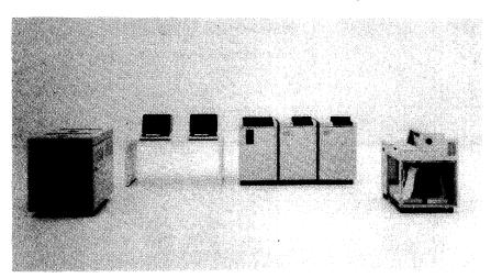
This IBM 8100 configuration includes, from left to right: two 8809 Magnetic Tape Units, two 8775 Display Terminals; an 8100 Processor, two 8101 Storage and I/O units, and a 3289 Line Printer, Model 3. An 8100 system can support up to 2,048K bytes of memory and 639 megabytes of disk storage.
