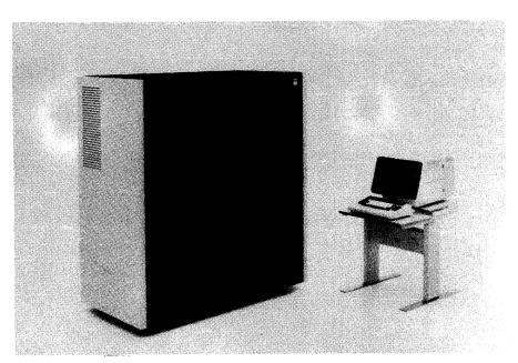
At the left is a picture of the 4381 processor and console which features from 4 to 16 megabytes of main memory, 4K to 32K bytes of buffer storage, and up to 12 I/O channels. It can utilize virtually all of the System/370 communications and peripheral equipment, including the high-performance 3380 Direct Access Storage Device. The 4381 supports the MVS/XA operating system as well as OS/VS1, and DOS/VSE.
