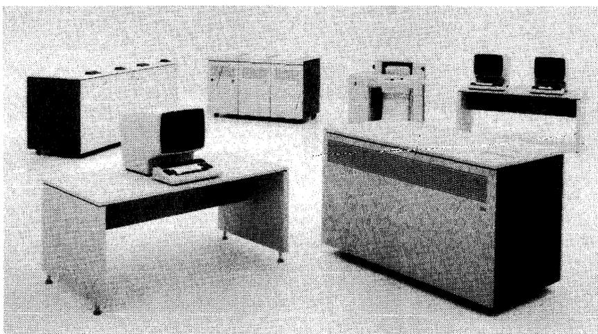
The 4331 Model Group 1 processor, at right foreground, is compact enough to fit easily into an office environment. The required 3278 Model 2A Display Console is in the left foreground, and behind it are four 3310 Direct-Access Storage Devices with a capacity of 64.5 megabytes each.
