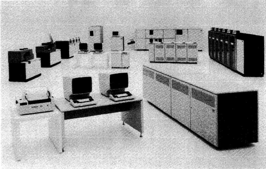
The IBM 4341 processor (right foreground) is priced below the System/370 Model 138 and delivers up to 3.2 times the CPU performance. It can utilize virtually all of the System/370 peripheral and communications equipment, as well as a number of devices introduced with the 4300 Series.
