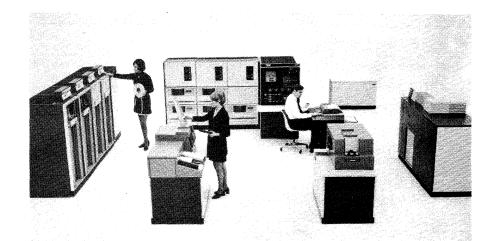
This Model 135 configuration includes a 5-drive disk storage subsystem attached directly to the central processing unit at center rear. In the foreground, from left to right, are the 3803/3420 Magnetic Tape Subsystem, 3505 Card Reader, 3525 Card Punch, and 3211 Printer.
