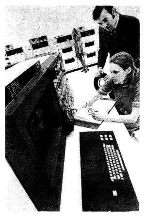
The largest of IBM's virtual storage computers, the Model 168 and its enhanced successor, the Model 168-3, offer up to 8 million bytes of real MOS main storage. A dual-processor Model 168 MP system can include up to 16 million bytes. The Model 168-3, announced in March 1975, features a 5 to 13 percent increase in instruction execution rates and a new Service Processor that expedites on-line error analysis.
