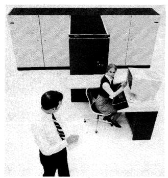
The System/370 Model 158 Processing Unit provides up to 2 million bytes of MOS main storage and up to 16 million bytes of virtual storage. A feature of the Model 158 is its CRT display console with light-pen input. The improved Model 158-3, introduced in March 1975, provides enhanced internal performance, additional reliability features, more flexible multiprocessor configurations, and expanded I/O subchannel capabilities.
