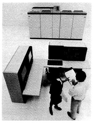
The Model 168, largest of IBM's virtual-storage computers, offers up to 8 million bytes of real MOS main storage; a dual-processor 168 MP system can have up to 16 million bytes. The Model 168 console features a CRT display and keyboard.
