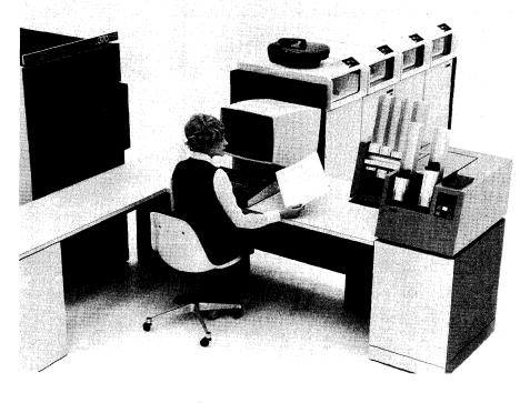
The Model 115, the smallest and newest member of the expanding System/370 family, employs distributed processing techniques and features integrated control units for attachment of disk drives, magnetic tape units, card unit, line printer, and communications terminals.
