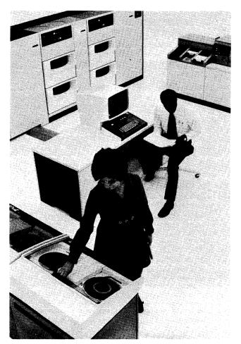
The Model 125, introduced in October 1972, was the first IBM system below the "super-computer" class to employ distributed processing techniques. Direct access storage devices available for the Model 125 include the 3330 Series Disk Storage drives (left rear) and the newer 3340 Direct Access Storage Facility.
