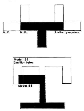
IBM's new MOS main memories result in greatly reduced floor space requirements. The top illustration shows a 2-million-byte Model 158 CPU (shaded black) superimposed against a Model 155 with the same amount of core storage. Below, a 2-million-byte Model 168 CPU is similarly compared with a Model 165 of equivalent capacity. standard I/O channels. The adapter occupies one control unit position on each of the two channels it interconnects.
