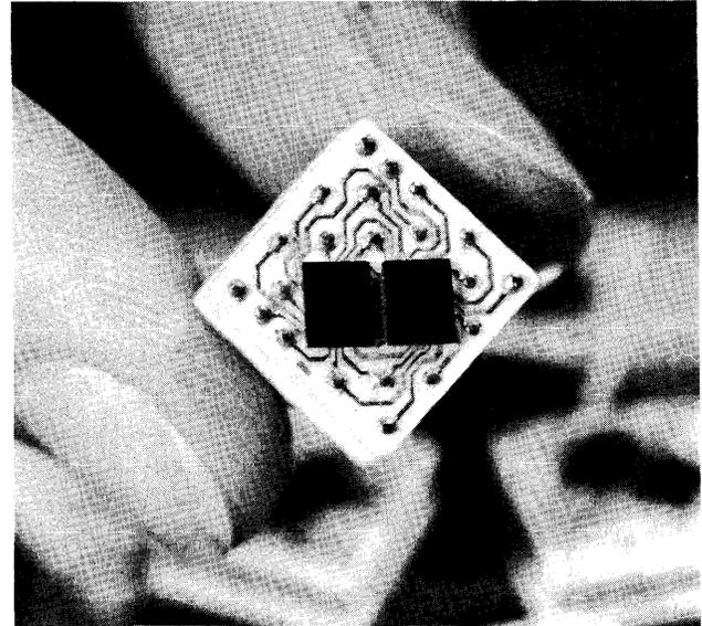
*Silicon chips, each about one-eighth-inch square, contain 1024 microscopically small MOS data storage circuits for use in Models 158 and 168. Two of the chips are shown here mounted on a ceramic base, which is assembled into a tiny 4-chip storage module containing 4096 circuits.*
