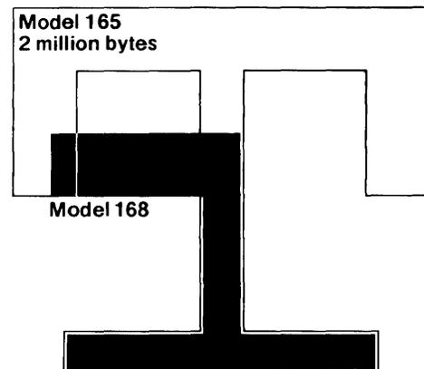
IBM's new MOS main memories result in greatly reduced floor-space requirements. The top illustration shows a 2-million-byte Model 158 CPU (shaded black) superimposed against a Model 155 with the same amount of core storage. Below, a 2-million-byte Model 168 CPU is similarly compared with a Model 165 of equivalent capacity.
