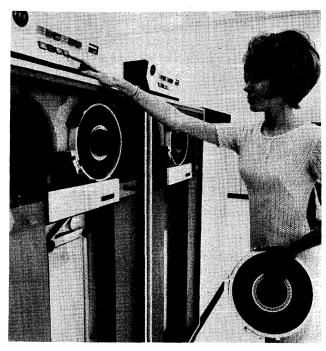
The IBM 3420 Magnetic Tape Units, introduced in November 1970, provide high performance (up to 320,000 bytes per second) at far lower prices than previous IBM tape drives.
