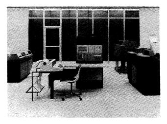
A disk-oriented System/360 Model 25 configuration.
