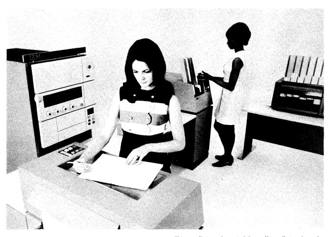
This overall view of a typical System/3 installation shows the 5203 Printer in the foreground, the off-line 5486 Card Sorter at far right.
