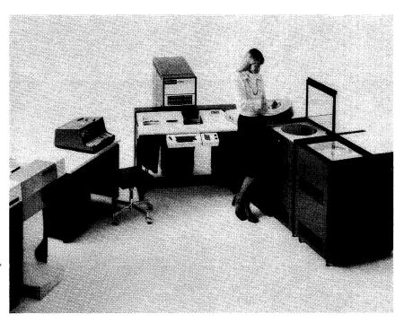
The Model 61/60 Transaction Processing System in its minimum configuration consists of the central processor with 10,240 bytes of memory; a front-end processor with its related 8K-byte memory, CRT display, keyboards, and two cassette tape units; a 100-lpm, 128-position printer; a card console consisting of a 100-cpm card reader, numeric keyboard, alphanumeric keyboard, and 10-digit display; and a mass storage subsystem with 46 megabytes of disk storage.
