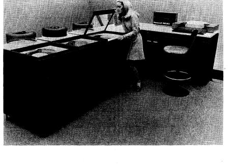
The Model 62/60, smallest member of Honeywell's new Series 60 computer family, is a disk-oriented system aimed primarily at new users. It offers from 65K to 131K bytes of 1-microsecond MOS memory. System rental prices range from approximately \$4,000 to \$7,000 per month.
