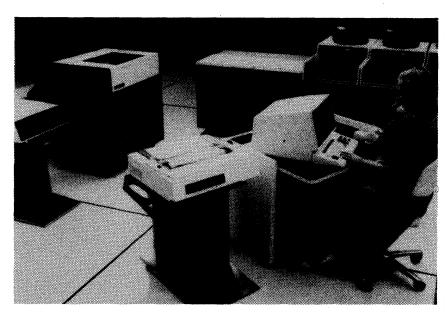
A typical DPS 7 configuration includes the operator console and printer plus (left to right) a diskette drive, high-speed line printer, the DPS 7/45 central processor, and three disk drives. The DPS 7 has from one to four megabytes of memory, and supports a wide variety of peripheral devices.
