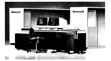
Honeywell's new top-of-the-line DPS 90 mainframe family includes one-, two-, three-, and four-processor models, plus a fully-redundant dual system. The top-end DPS 90/94 can be configured with up to 256 megabytes of main memory and delivers three times the processing power of the DPS 88, Honeywell's previous top-end series.
