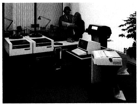
Providing a natural growth path for Level 61 users, the DPS 4 fits easily into the normal office environment: the set of processors is housed in a 144 cm by 50 cm by 76 cm cabinet.
