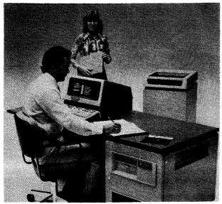
This picture of HP's new 3000 Series 33, based on silicon-onsapphire technology, clearly shows the compactness resulting from the SOS/CMOS circuits. The desk contains the CPU, 256K bytes of fault-control memory, seven terminal ports, two general I/O channels, and a 250K-byte floppy disc unit. The 50-megabyte system disc stands behind the desk. All Series 33 software is compatible with the larger HP 3000 Series II and III systems running under MPE III.
