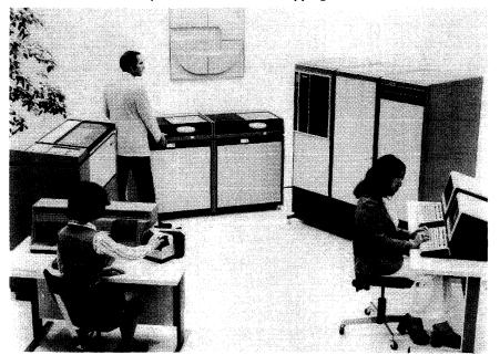
Pictured here is the largest model of the 3000CX family, the 300CX. Features include virtual memory, stack architecture, and dynamic resource allocation. This model also supports a data base management package, along with FORTRAN, BASIC, ANSI COBOL, RPG II, and SPL (Systems Programming Language).
