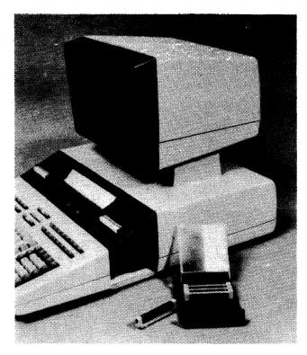
Hewlett-Packard's System 45 allows the addition of up to 16 readonly memories (ROM's) that fit into two drawers found on the sides of the desk-top computer. One such ROM is shown in the lower center of the picture, and three more are in the storage case to the right. The modules are 0.4 x 3.8 x 1.1 inches and weigh 1.4 oz.
