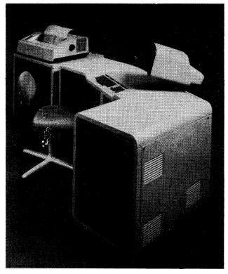
The basic HP 250 consists of an operator's console with keyboard and adjustable display screen (center) and disk storage (right), all housed in a compact desk enclosure. The system shown also includes (left) a 2631A serial printer.
