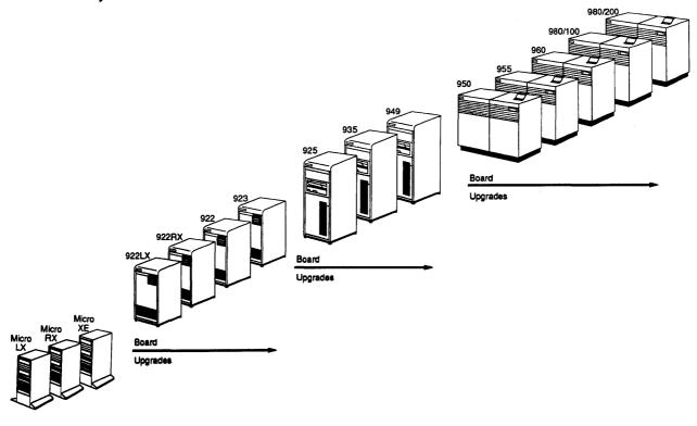
The HP 3000 family simple board upgrades provide a growth path within each level of the HP 3000 Series 90.
