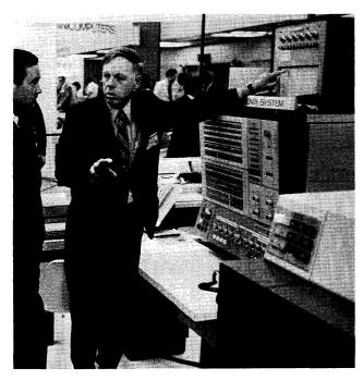
The Phoenix X-30 console will be comfortingly familiar to anyone who has operated an IBM 360/30. Atop the CPU cabinet is a multiple-pen chart recorder that was used to measure and analyze the system's performance on live benchmark tests at the National Computer Conference.
