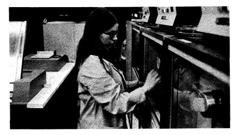
Phoenix System buyers can elect to use magnetic tape units and disk drives manufactured by either IBM or CalComp. Punched card I/O functions will normally be handled by the familiar IBM 2540 Card Read Punch at left.
