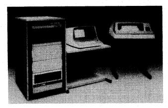
The above Solution system, based on the GA-16/240 CPU, includes a 10-megabyte cartridge disk drive, a general-purpose display terminal, and a 300-lpm printer. The purchase price for this system, including 128K bytes of memory, is about \$31,100.
