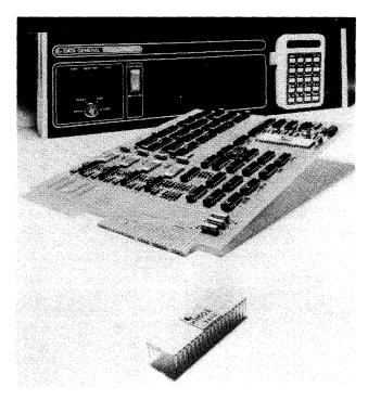
The microNova family consists of three basic configurations: chip sets, board computers, and fully packaged microNova minicomputers. Recent hardware offerings include graphics terminals, graphics printers, and intelligent terminals.
