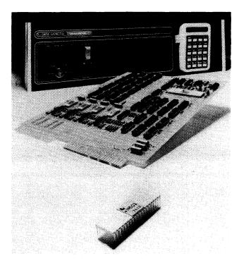
The microNova family is available in three basic configurations: chip sets, board computers, and fully packaged microNova minicomputers. All the packaged variations are built around the 40-pin mN601 NMOS microNova processor (foreground), which features a full 16-bit Nova architecture and main memory addressing capacity of up to 32K words.
