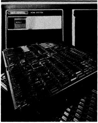
The two-board design of Data General's Nova<sup>®</sup> 4/X computer incorporates CPU, MMPU, async interface, real-time clock, automatic program load, and power fail/auto restart on the CPU board, and up to 256K bytes of memory on a single memory board.
