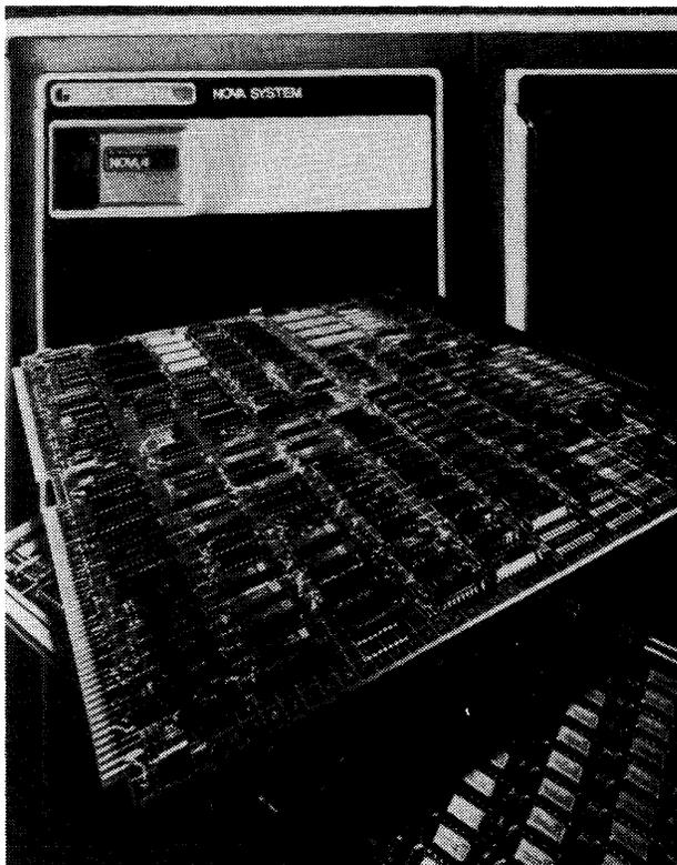
The two-board design of Data General's Nova® 4/X computer incorporates CPU, MPPU, async interface, real-time clock, automatic program load, and power fail/auto restart on the CPU board, and up to 256K bytes of memory on a single memory board.
