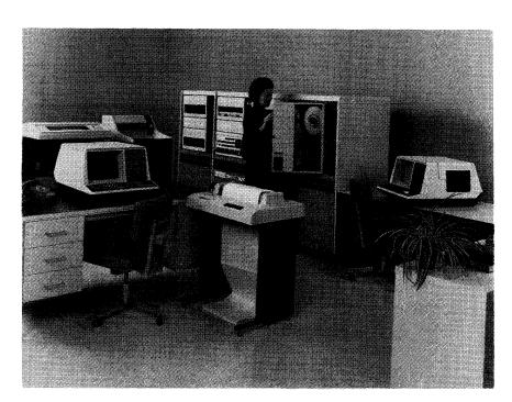
Utilizing the PDP-11/34, 11/60, or 11/70 processor, the DEC Datasystem 500 family supports a maximum of 64 terminals, 2040K bytes of core memory, and up to 4 billion bytes of disk storage. The configuration shown includes a 176-megabyte disk drive, a VTS2 terminal, a 300-lpm printer, a 1600-bpi magnetic tape transport, and a DEC writer hard-copy terminal.
