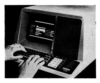
The new forms-oriented VT62 display terminal for DEC's TRAX system includes reverse video display, automatic cursor positioning, error detection features, and special message displays. PDP-11/70 TRAX systems can support up to 64 VT62 terminals.
