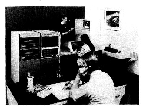
≥ above peripherals can also interface with the Unibus, and still work at their normal speeds. (The special PDP-11/70 fast bus and fast controllers for these peripherals serve only to assist the central processor.)
