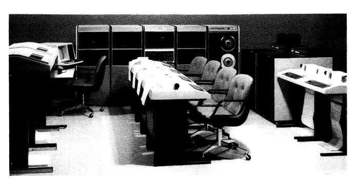
The newest DEC Datasystem, the 570, is an on-line multiterminal system based on the new DEC PDP-11/70 and announced with the new processor in February 1975. The congiguration shown here includes (from left to right, in the background) a pair of 132-position 300-lpm DEC LP11 line printers, a VT50 DECscope display terminal and keyboard, a PDP-11/70 with 192K bytes of
