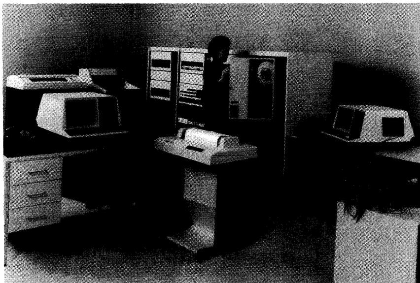
*Utilizing the PDP-11/23, 11/23-PLUS, 11/24, 11/44, 11/34A or 11/70 processor, the DEC Datasystem family supports a maximum of 127 terminals, 3.5 megabytes of memory, and up to 1.4 gigabytes of disk storage. The configuration shown includes a 176-megabyte disk drive, a VT100 terminal, a 300-lpm printer, a 1600-bpi magnetic tape transport, and a DECwriter hard-copy terminal.*
