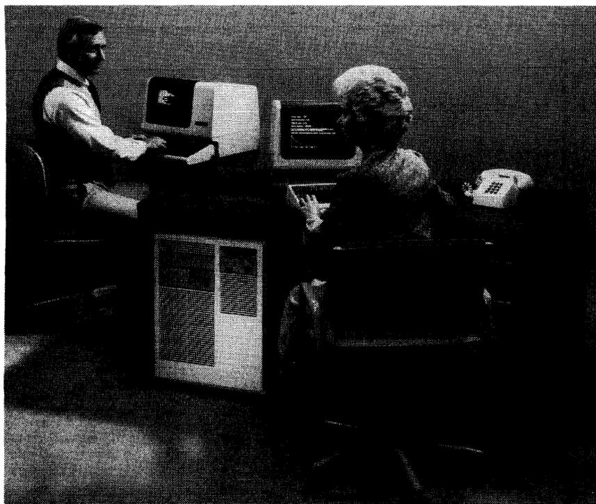
*The new VAX-11/725 supermini-computer is Digital Equipment Corporation's smallest, least expensive Unibus-based VAX system, featuring quiet operation and low heat generation for open-office environments. With a VAX-11/730 processor and the new, high-capacity RC25 52MB fixed and removable 8-inch Winchester disk subsystem, the VAX-11/725 serves as a low-cost, multiuser system for general-purpose applications or as a computing "engine" for high-performance graphics workstations.*
