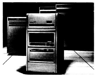
The newest member of Digital Equipment Corporation's VAX family of virtual memory computers is the VAX-11/730, shown above in a single, 42-inch high cabinet with 131 megabytes of fixed and removable disk storage. Other VAX systems pictured are the mid-range VAX-11/750 (left), VAX-11/780 (right), and the VAX-11/782 attached processor system (rear). Prices range from \$48,900 for an entry-level VAX-11/730 package to \$445,000 for the top-of-the-line VAX-11/782 package.
